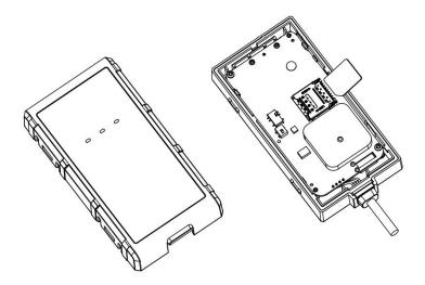
4. To ensure waterproof take effect, make sure the silicon rubber ring is installed in place.
