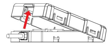
3. Insert SIM card into the slot and toggle the switch to ON.
