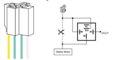
12V relay is standard. The device is suitable for vehicles with 12V supply. If the vehicle power supply is 24V, use 24V relay.
