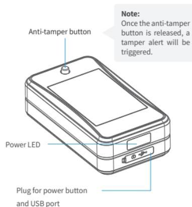
**Note:** Once the anti-tamper button is released, a tamper alert will be triggered.
